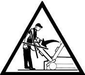
Keep at a safe distance during tilting of the tool head in order to avoid crushing.
