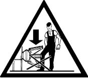
During descent of the self-centring device, whether with the wheel fitted or with the device open, keep at a safe distance to avoid the risk of crushing.
