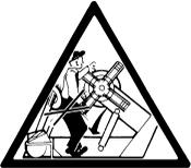
NEVER get between the tool head and the rim or wheel secured on the spindle.
