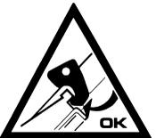
Before carrying out any operation with the tools, make certain that the arm locking hooks are completely fastened.
