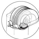
Do not lift up the guard when the wheel is turning.
