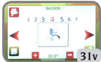
Wheel rotation activates automatically in order to complete extraction of the top bead.
