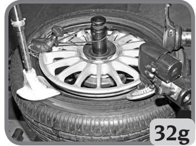
Proceed with mounting the top bead using the bead presser (Fig. 32f) and, if necessary, the bead presser pliers (Fig. 32g).
