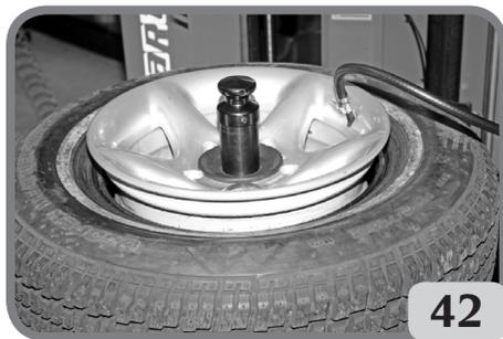
Step down partially on the pedal to inflate the tyre and seal beads with the inflation hose. Frequently stop to check bead seating pressure on the gauge.
