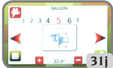
Wheel rotation and ascent of the bead breaker disc activates automatically in order to complete extraction of the bottom bead.
