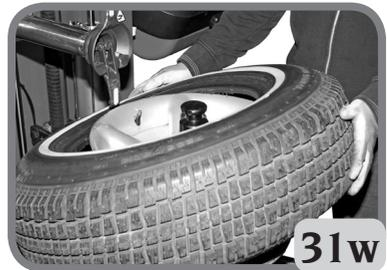
**Demounting the bottom bead using the demounting tool and bead breaker.**
