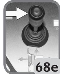
6. Operate the lever to position the upper bead breaker downwards until the lower part of the bead breaking disc is aligned with the upper surface of the template (see Fig. 68f).
