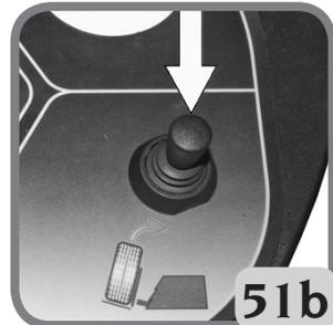
Operate the Lever (Fig. 51b) and lift the wheel from the wheel support plate (Fig. 51c). Move the wheel to the left, until it rests on the frame (Fig. 51d).
