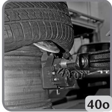
17- If necessary, operate the control to slightly lift the lower bead breaker.
