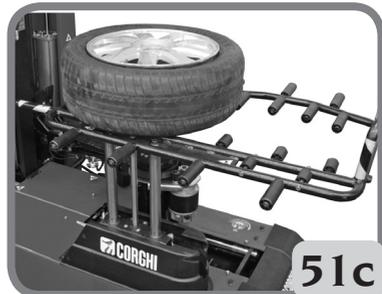
Continue to operate the Lever until the lifter is on the ground (Fig. 51e). Unload the wheel from the lifter and move it away from the work area.
