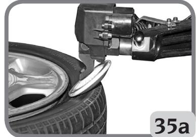
5 - Operate the control
