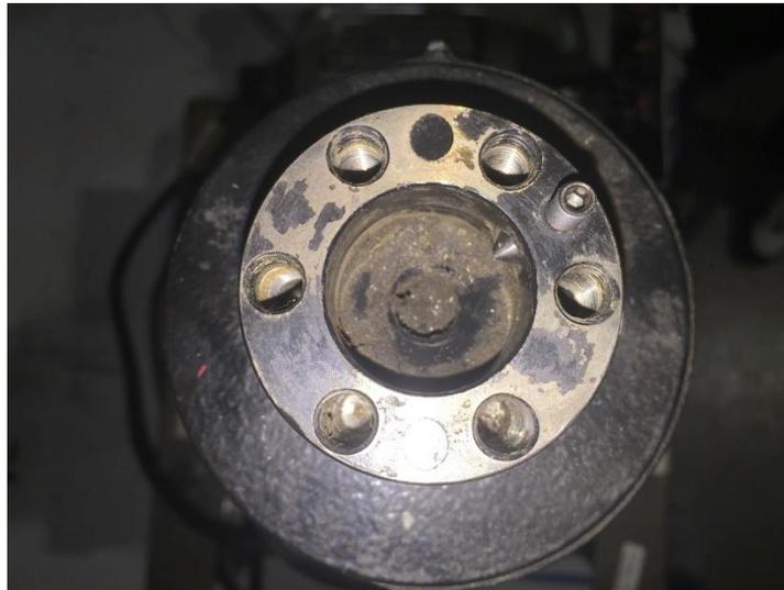
3. Place the Lock Plate on top of the transmission so that the Lock Screw is in one of the smaller holes. Insert two of the Turn Table bolts to hold the lock plate in place. In order to operate correctly, the flat surface of the Stop Screw must be parallel with one of the flats in the center of the Lock Plate as shown.
