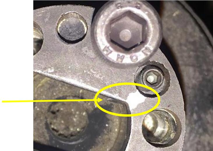
4. To adjust the stop screw, place the pistol shaft through the lock plate. When the pistol shaft is rotated clockwise it must rotate a full 90 degrees. If it does not, you have the plate installed incorrectly. When the pistol is rotated counterclockwise and engages the Stop Screw it should pull straight out. Screw the Stop screw in or out until you are able to insert and remove the pistol smoothly.
