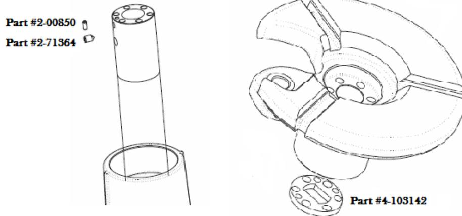
1. Remove the Turn Table, Lock Plate (4-103412), Stop Lock Screw (2-00850), and the Pistol Stop Screw (2-71364).
