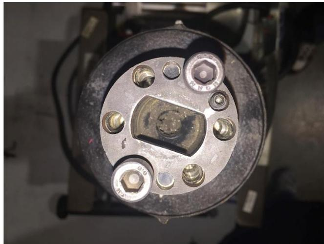
5. Once you have achieved smooth operation. Tighten the Stop Lock Screw. Remove the two turn table bolts and install the turn table. Double check correct operation of the pistol.
