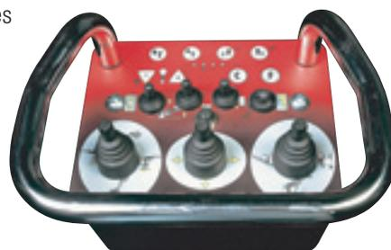
The **new controller with very handy controls** enables efficient operation of the tyre changer without the operator **touching the tools.**
