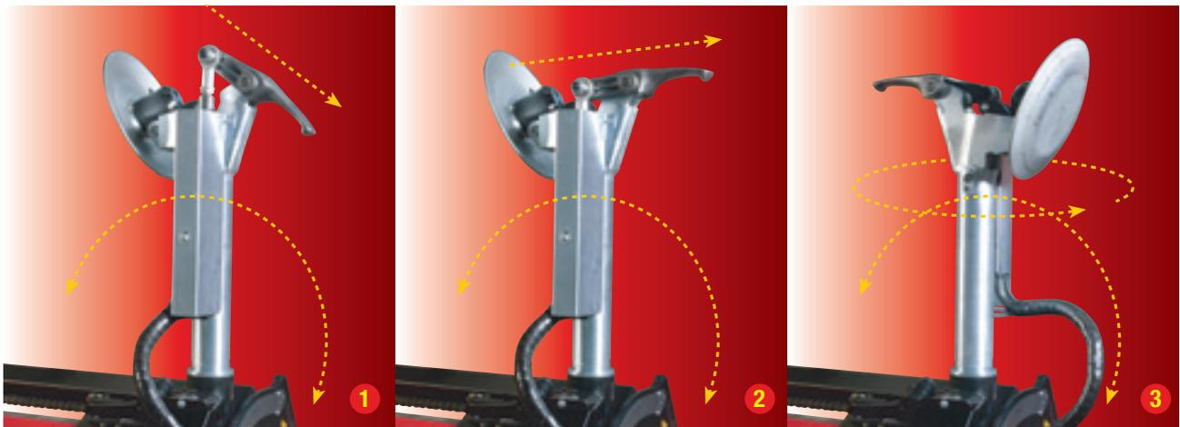
Sequence of automatic movements of the bead loosener disc:
