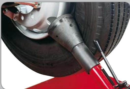
Demounting by means of roller
