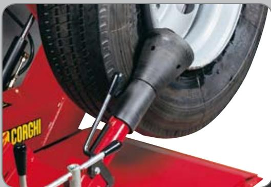
Bead breaking on outside of tyre
